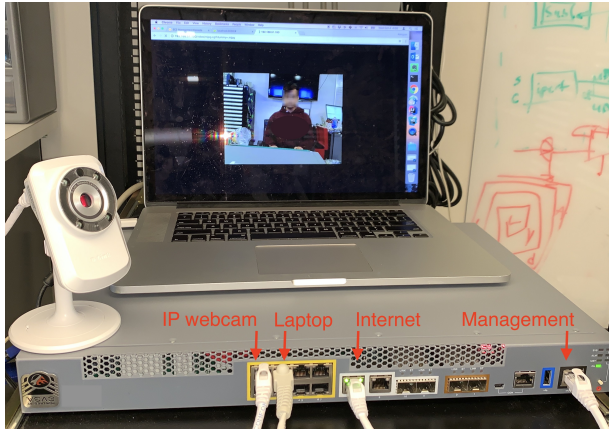
Figure 3. Demo of a face blurring VNF (running on AWS EC2) processing video stream from a customer premise equipment.
